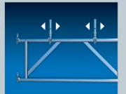
Variable - The width and position of the scaffolding can be variably adjusted.
