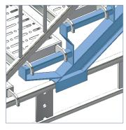
Individual: The lower support of the stair stringer is positioned directly on the ledger. This means that the same ledger can be used for all stringer heights. The system is completed with steel decks or planks for tube hook-up.
